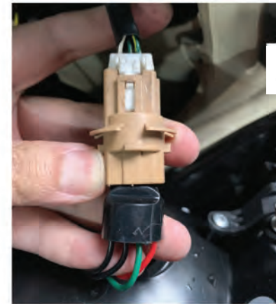
Insert the harness socket of the retrofit light into the socket (no need to distinguish between positive and negative).
