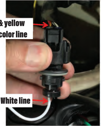
Pay attention to the reverse lights. (The white line on the light body corresponds to the red and yellow two-color line on the car body).
